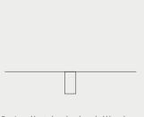
1. A pilot hole is drilled and a tapped metal plug is fixed in the deck.
